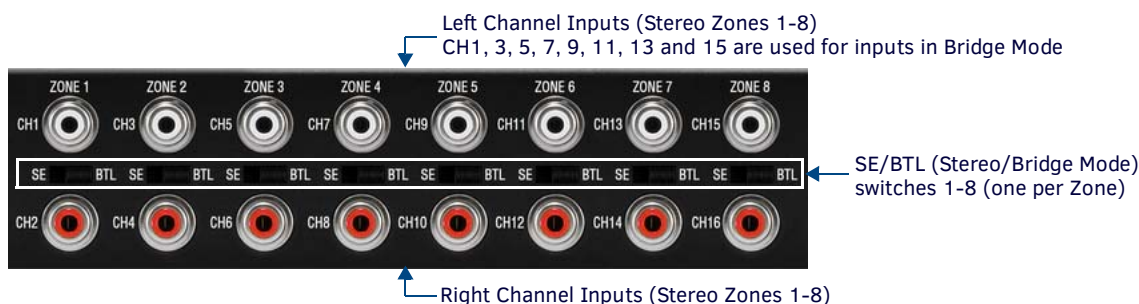
FIG. 4 Audio Input connectors (L/R pairs for 8 stereo inputs, 16 total)
