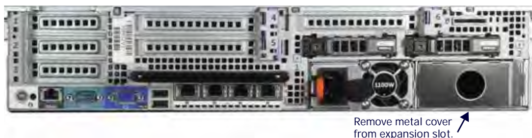
FIG. 8 Master Server Rear Panel
