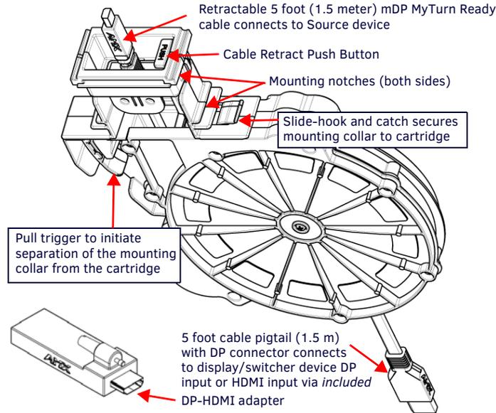
**FIG. 1** HPX-AV102A-MDP-R MINI-DISPLAYPORT MODULE WITH RETRACTABLE CABLE
