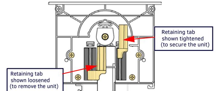
FIG. 11 HPX BASE ASSEMBLY (SHOWN MOUNTED) - MOUNTING SCREWS LOCATIONS
