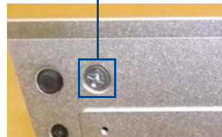
FIG. 3 LOCATION OF THE PHILLIPS HEAD SCREWS ON THE BOTTOM OF THE TOUCH PANEL
