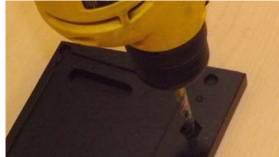
FIG. 2 MARKING THE LOCATION OF THE HEX HEAD BOLT HOLES
