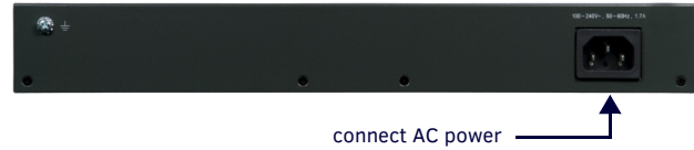
FIG. 2 PLUG THE AC POWER CORD INTO THE SOCKET ON THE REAR OF THE SWITCH
