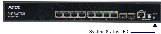
FIG. 3 SYSTEM STATUS LEDs
