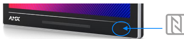
FIG. 7 NFC Sensor Location & Decal Placement
