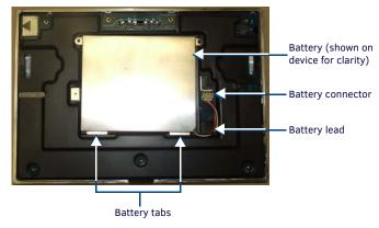
FIG. 4 INTERIOR OF MVP-9000I, INCLUDING FEMALE BATTERY CONNECTOR
