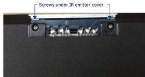
FIG. 2 PLACEMENT OF SCREWS UNDERNEATH IR EMITTER COVER
