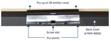
FIG. 1 IR EMITTER COVER REMOVAL
