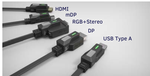
FIG. 6 MYTURN-READY SOURCE SELECTOR BUTTONS SHOWN MOUNTED ON VARIOUS CABLES
