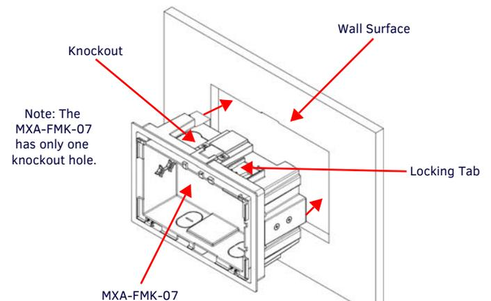
**FIG. 3** INSERTING THE MXA-FMK-07 INTO THE WALL SURFACE (LANDSCAPE)
