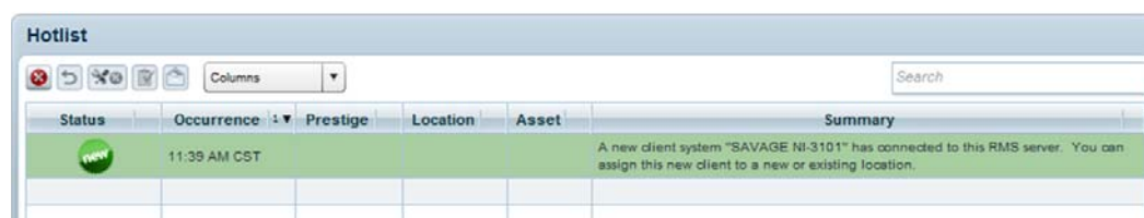
FIG. 18 RMS Hotlist - Newly Registered Client Gateway
