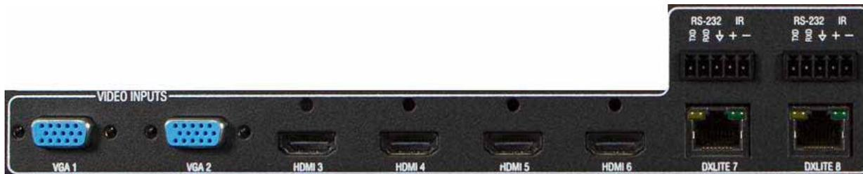
FIG. 27 VIDEO INPUTS ports
