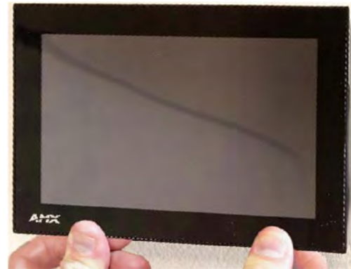
FIG. 8 LOCKING DOWN THE BOTTOM OF THE TOUCH PANEL ONTO THE BACK BOX.
