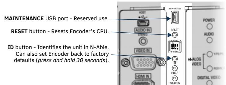
FIG. 3 BUTTONS LOCATED ON FRONT-CENTER OF UNIT
